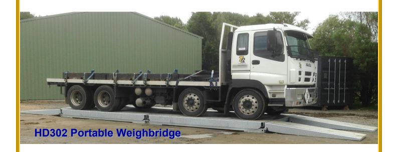
Hot dip galvanised or Epoxy paint finish
